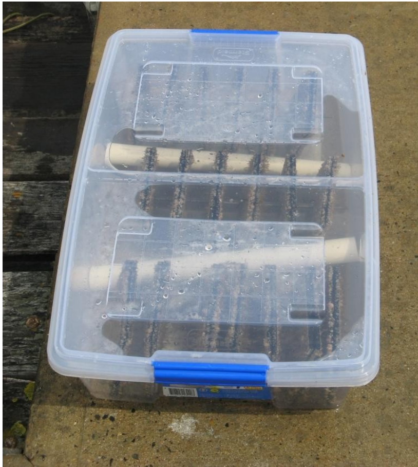
Plate 5. Recruitment plates held on stainless steel allthread with plastic tubing spacers to keep each set of plates separate. PVC tubing is used to separate the three allthreads of plates and the perfectly fitting container also holds them in place. Using this holding system enables the plates to be brought from the field by vehicle to the laboratory without any damage occurring to the recruitment assemblages. Plates were removed from the backing panels at Fisheries Wharf, Cronulla.
