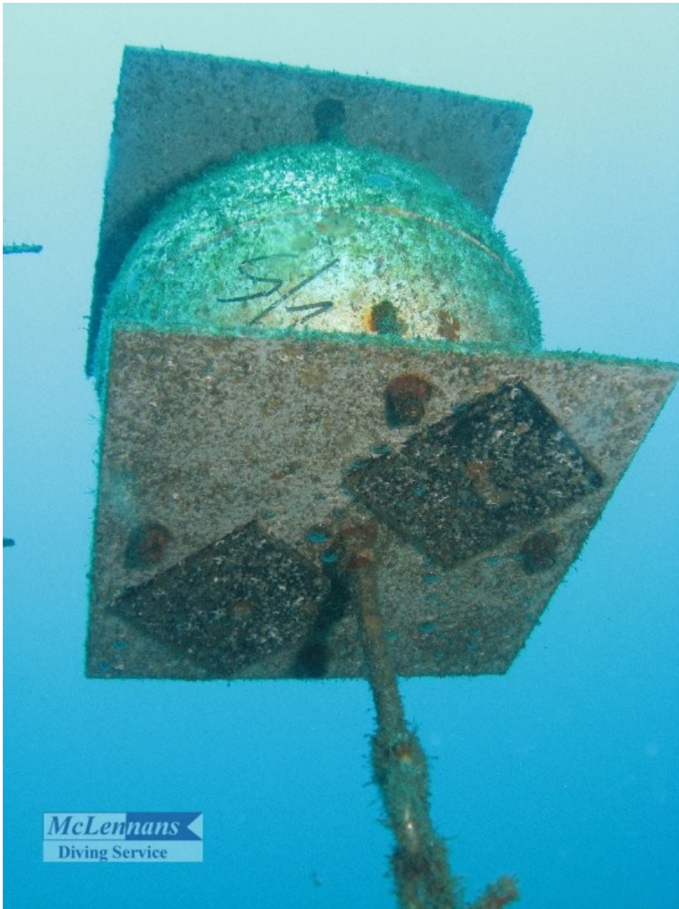
Plate 2. Two recruitment plates (roughened Perspex) attached to the downward surface of a panel/float. Four panels are set up in an array (a site) with 2 sets of arrays at each location (Photograph courtesy of McLennans Diving Services).
