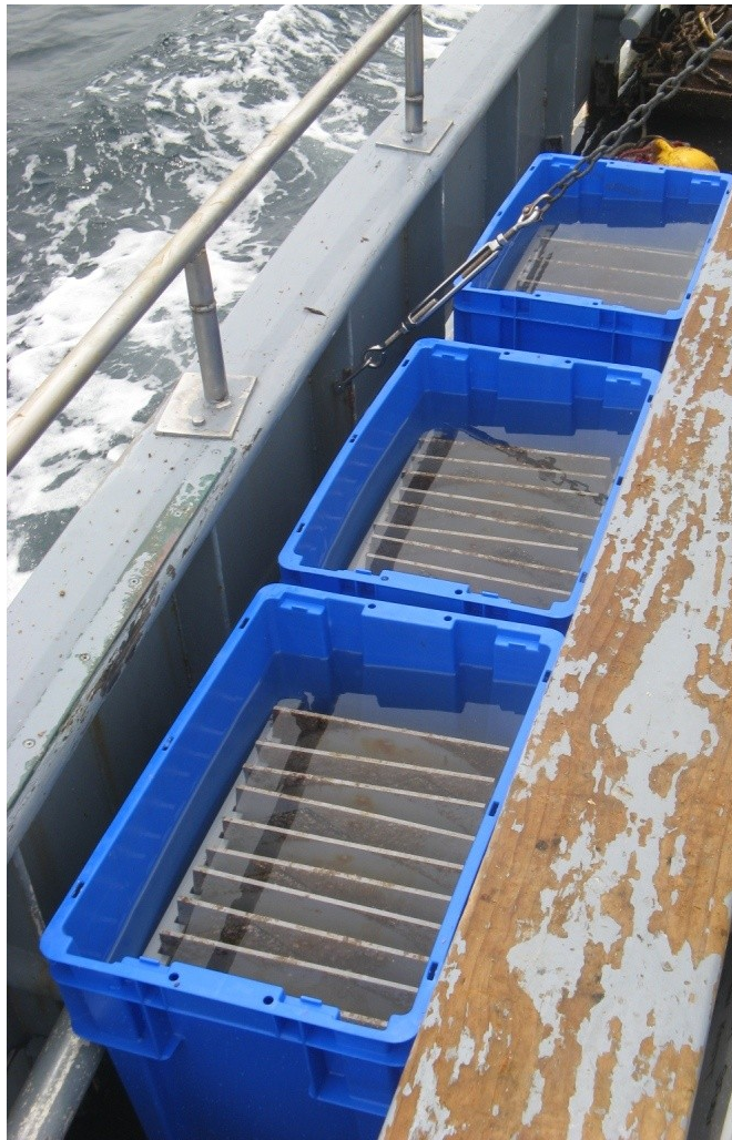
Plate 4. Recruitment plates attached to PVC backing panels held in specially designed frames to safely hold the samples during collection at sea.
